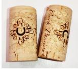
The **PLATINCORK** – **A** (PL 1+1 AGLO), is a recommended technical closure for wines with an expected consumption within an approximate period of 2 a 3 years. It is, therefore, an excellent option for bottling wines with a certain complexity and moderate rotation. Made up of a natural cork disc at both ends and an agglomerate body, this type of stopper offers excellent mechanical behaviour (torsion, dimensional recovery/elasticity) and excellent sealing capacity.
